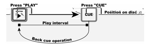
**PLAY and CUE:** Pressing the "PLAY" button starts the disc. Pressing the "CUE" button will reset the disc to the last place where the disc was started. This is called the cue point. By alternately pressing the "PLAY" button and the "CUE" button, the disc may be returned and played from the cue point any number of times. This function is called back cue.
